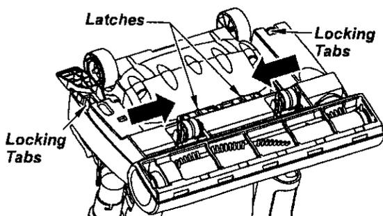
Locate the two latches and the two locking tabs which secure the base plate.
